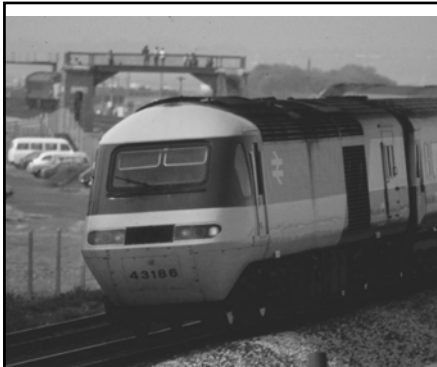
High Speed Train cab unit made from GFRP
