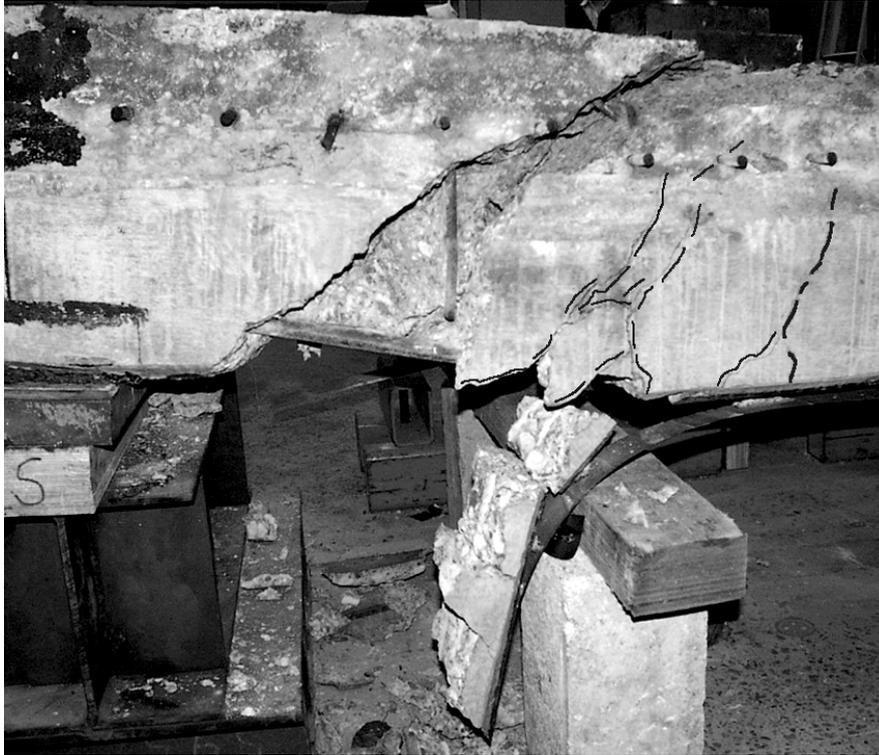
**Figure 5: Failure Showing Extensive Cracks And Peeling of Carbon Fibre Strap on West Side for Beam 3-3 from Bridge 4658**
