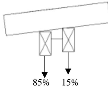
**Figure 6: Average Percentages of Timber Half-Cap Load Sharing Capabilities**
