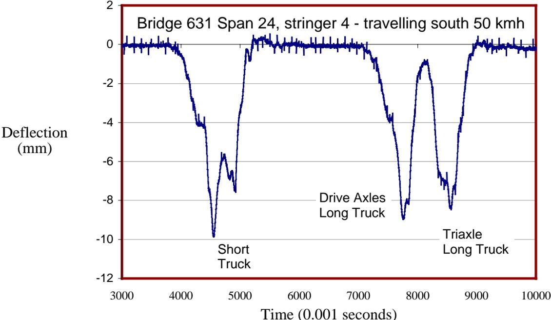
**Figure 2: Typical Dynamic Deflection Response for Bridge 631 – Trucks Travelling in Convoy**
