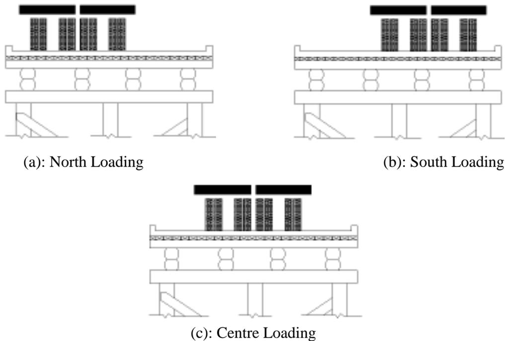
**Figure 5:** *Lateral Loading Positions of Truck across the Bridge Deck*
