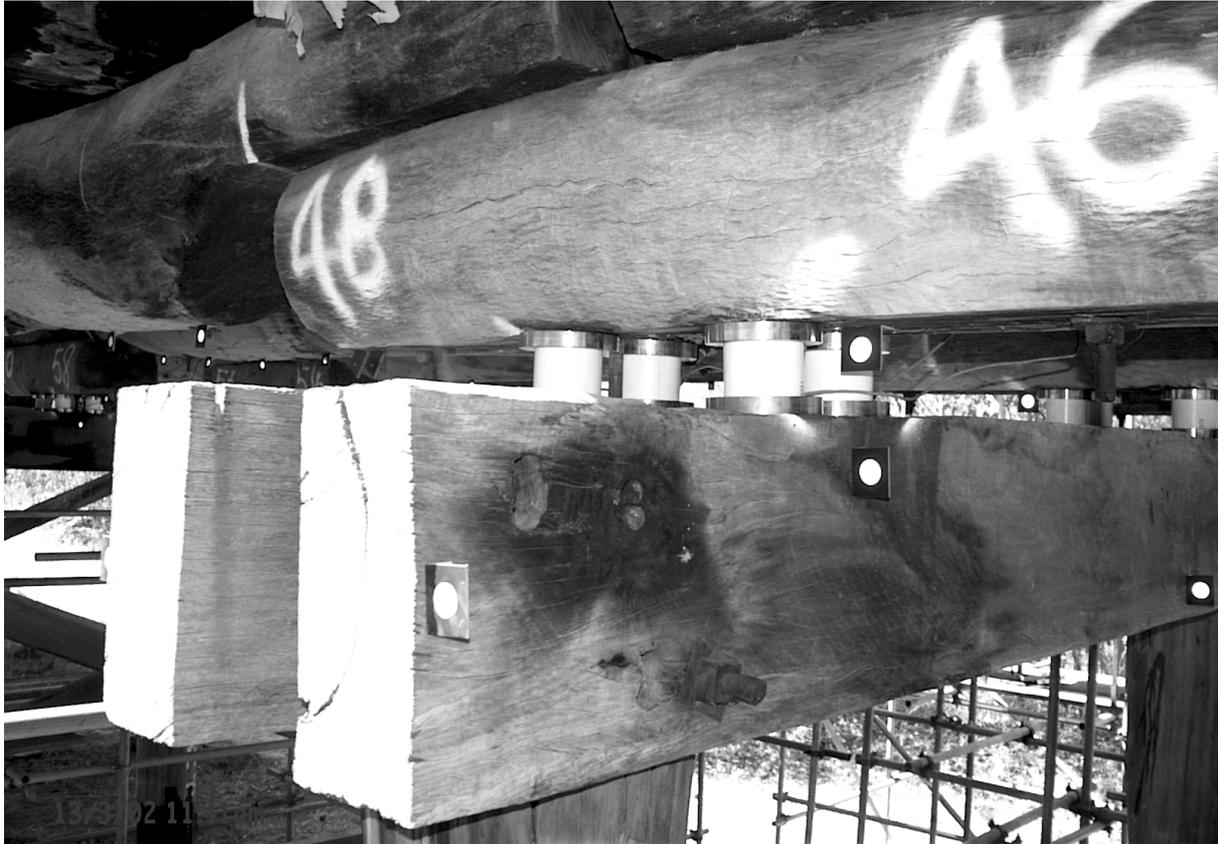
*Figure 4: Typical Arrangement of Four Loadcells Inserted between a Corbel and Halfcaps*
