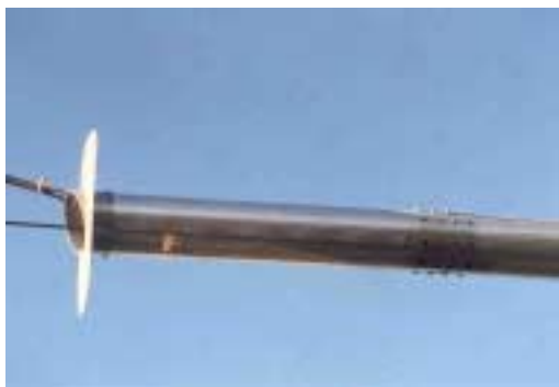
Fig. 16: Close up of perforated tube of fauna funnel showing entrance baffle.
