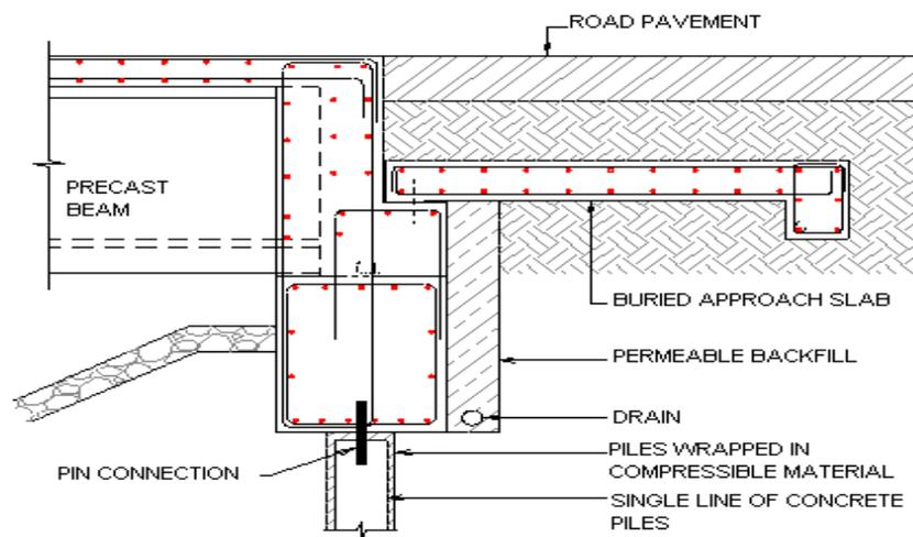
**Figure 7: Buried Approach Slab and Integral Abutment**
