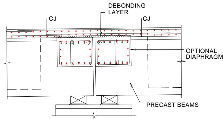
***Figure 1: Link Slab Detail at Intermediate Pier Locations***
