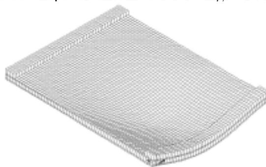
***Figure 2: Discretised End Span Model – Deflected Shape***
