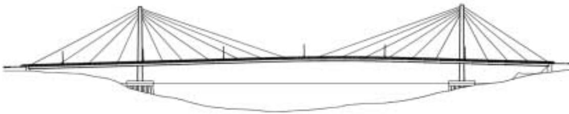
*Figure 5: Option 10 - Twin tower cable stayed bridge*
