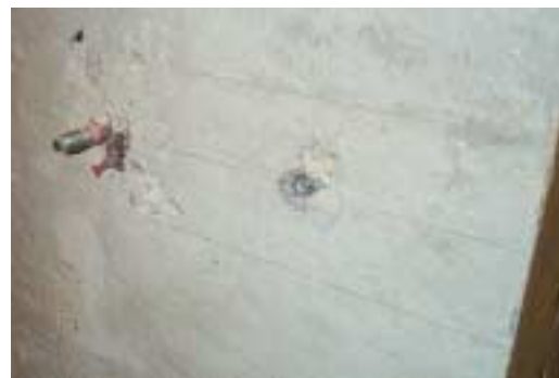
(a) concrete splitting (100 mm edge distance) (b) anchor bolt shear (125 mm edge distance)
