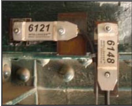
Figure 3: Transducers Measuring Slip and Separation
