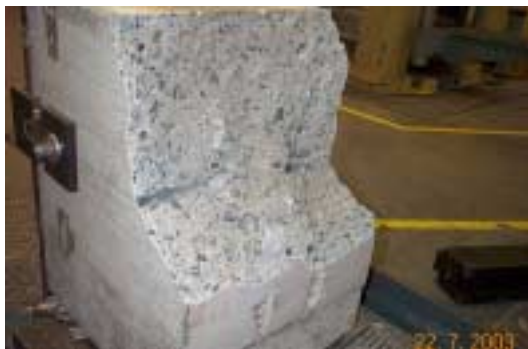
(a) concrete splitting (100 mm edge distance) (b) anchor bolt shear (125 mm edge distance)
