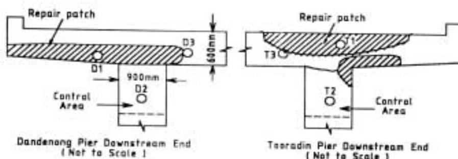
*Figure 1: Location of Ag/AgCl Reference Electrodes and Patch Repairs*
