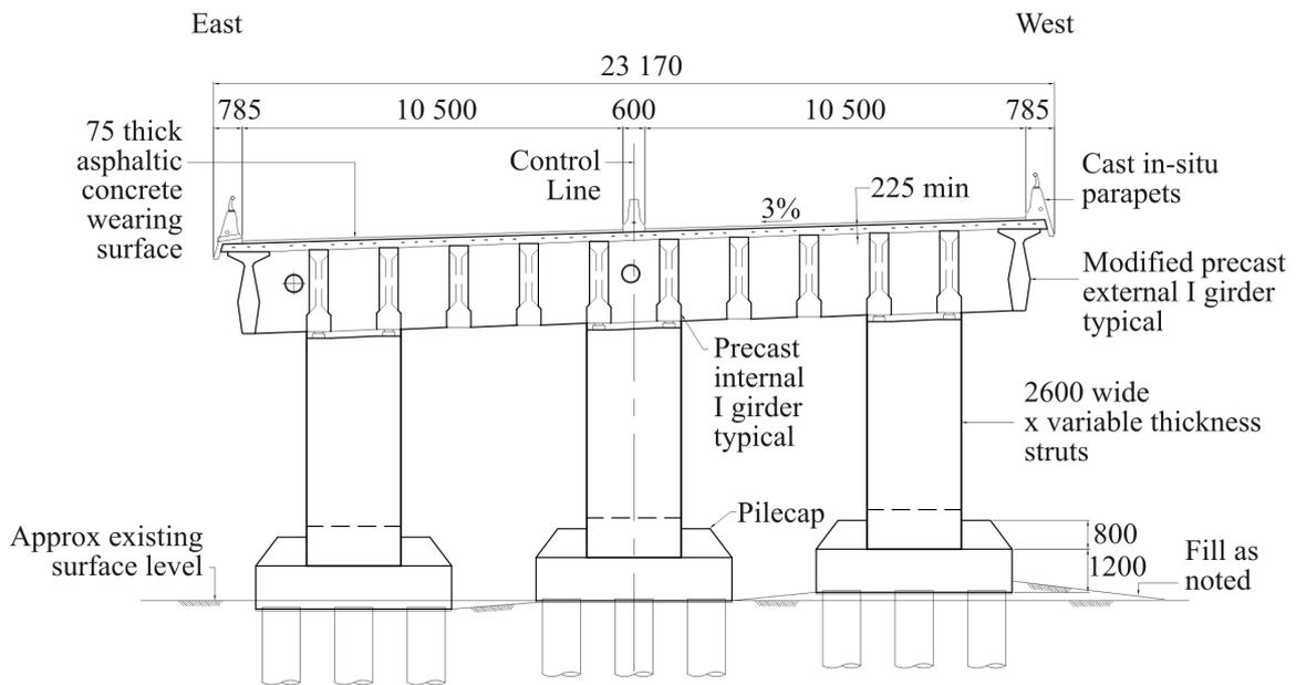
Figure 3: Main Span, Cross Section
