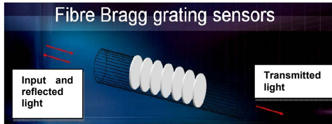
Figure 6: Workings of an FBG (Grattan et al. 2006)
