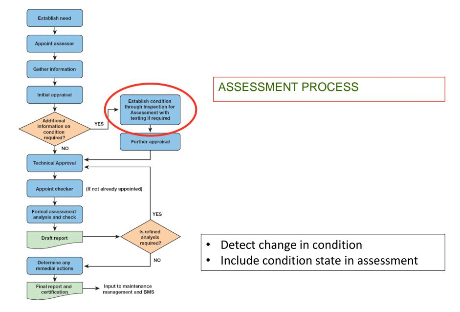
Figure 7.1: Flowchart of the assessment process for a highway structure
