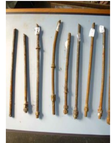
Missing studs found at Balcombe tunnel
