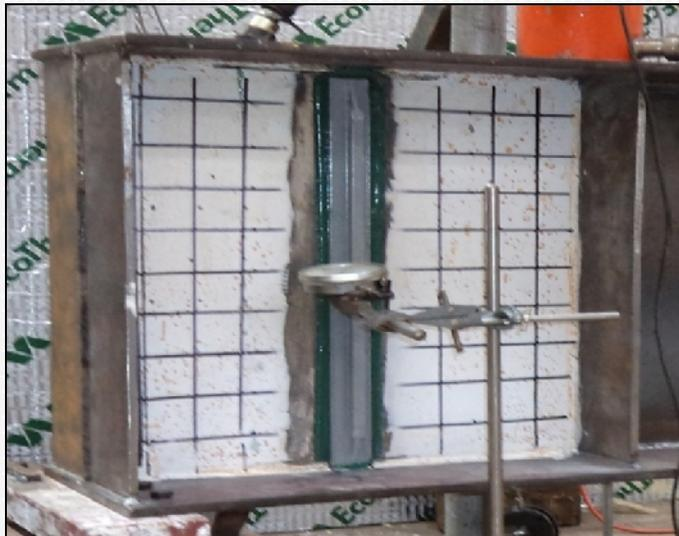
**GFRP-strengthened specimen B5**
