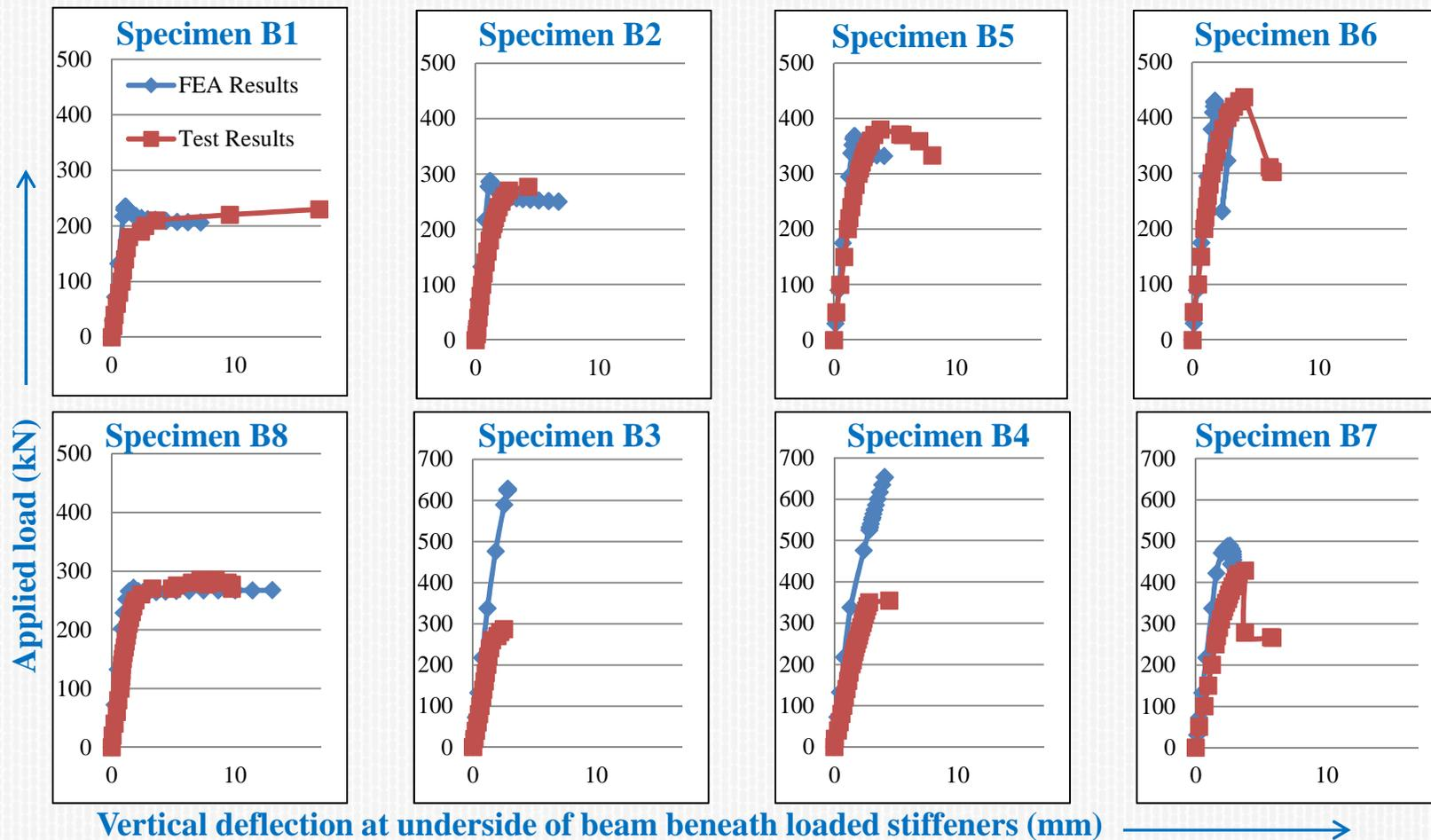
Note: The test and the FEA plots of specimens B3, B4 and B7 are not in good agreement because the FE analyses could not detect a bond breakdown of the steel-fabric bond that occurred in the tests
