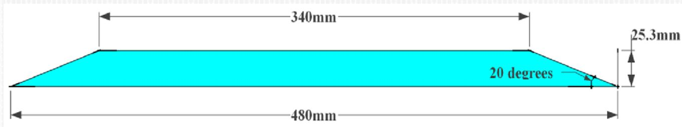
Side view of tapered GFRP stiffener of specimen B5
