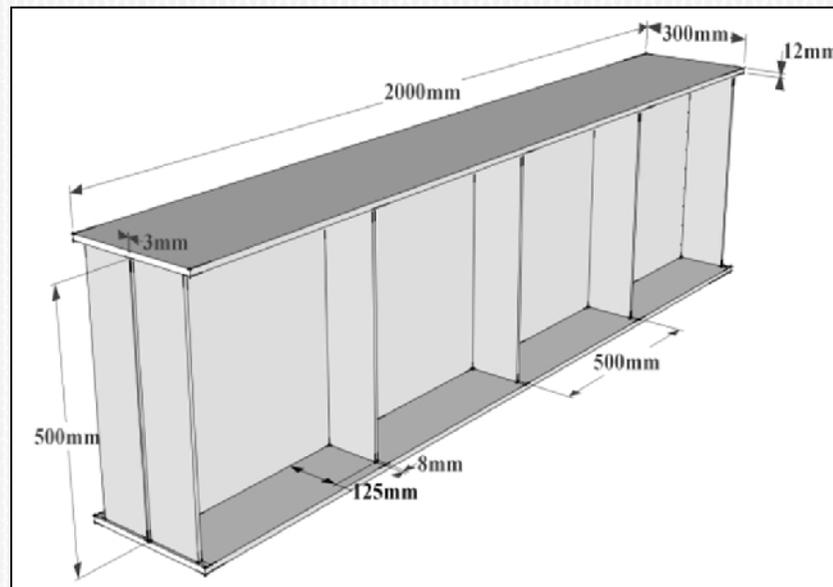
**S2 beam used for specimens B5 to B8**
