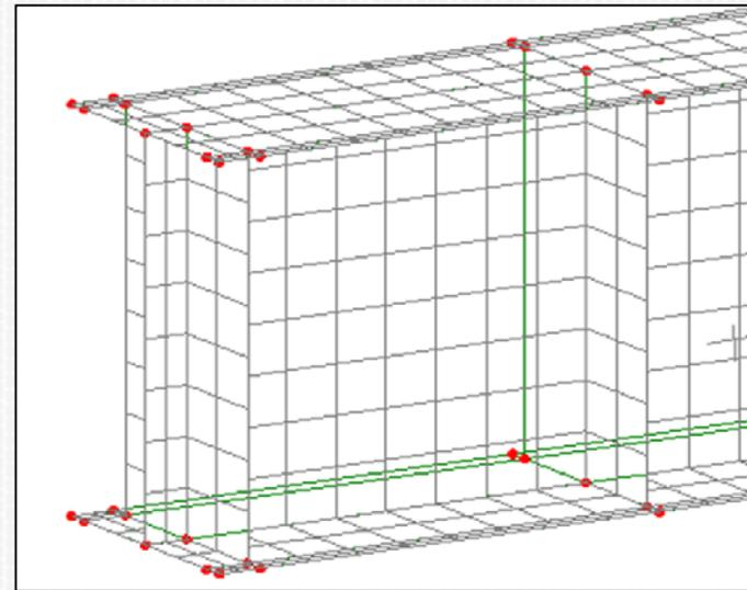
**Note: After a good agreement between the test and the FEA results of control specimen B1 for S1 beams, an FE model B9 was used as the control for S2 beams instead of a separate control test specimen**
