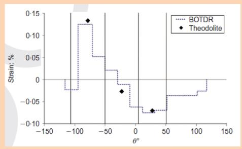
Displacement measurements will not tell if there is a problem Strain measurements will
