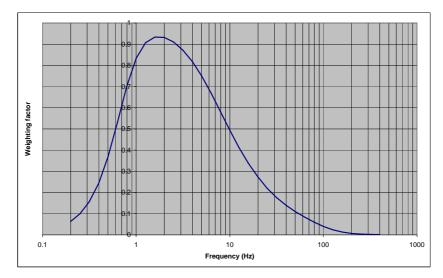
Figure 7: ISO 2631-2 frequency weighting factors
